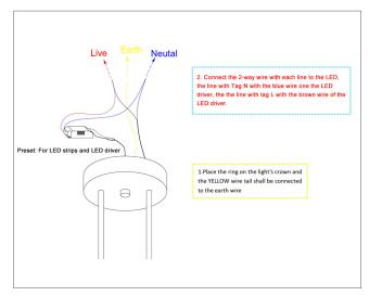
Step 6: As the above picture shown, then can finish the installation of wire, LED strips and driver.
