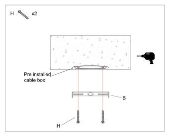
Step 5: Punch holes on the ceiling wall with an electric drill, insert the H through the B into the pre installed cable box and tide them finally.
