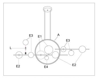
Step 9: Ensuring all bulbs (L) and LED light A are light, and fix up all the light shade (E) finally.
