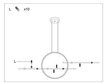
Step 7: After all the bulbs are installed, without the lamp shade wiring, test hanging, lighting up. If not light, it is suggested to re-check the wiring of the previous step. If you need a help, you shall take a picture about the wiring situation and then contact our after-sales service.
