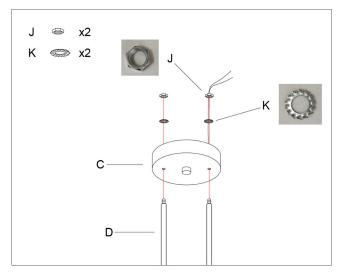
Step 4: Use the nut to lock C and D together.
