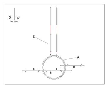
Step 3: Put the wire on A through D and twist D to fix it on A.
