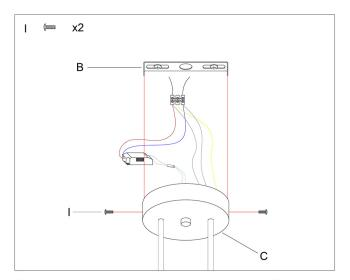
Step 8: Insert the screw (I) into the canopy (C) and fix it on both ends of B.
