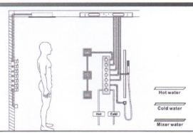
Schematic diagram of waterway installation
