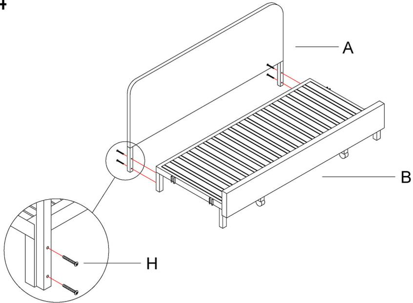
For all steps, align the holes first, then tighten the bolts
