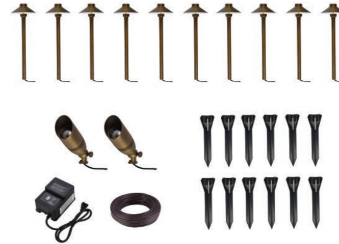
Model: KIT40210 Landscape Set 2Spot 10Path 12Spike 1Tran & Wire Spot light D:2 1/4" H:4 7/8" Path light D:6" H:18 1/8" LOW VOLTAGE LANDSCAPE TRANSFORMER 120W, INPUT: 120V,1.2A OUTPUT: 12V AC A roll of 100ft SPT2-16 wire Finish: Antique Brass
