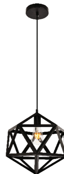
Model: LDPD2110 Diameter: 13" Body Height: 14.5" Overall Height: 21" to 74"(Adjustable) Wire: 60" Canopy Size: D4.7"*H1" Fixture Weight (LBS): 2.6 Light: 1 Type of bulb: Medium base (E26) Max Wattage: 40W (each bulb) Finish: Black
